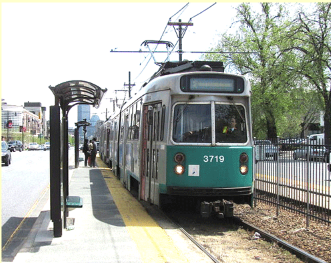
One of Boston's (MBTA) 120 KinkiSharyo Type 7/7.5 low floor vehicles on The Boston College or "B"line!
